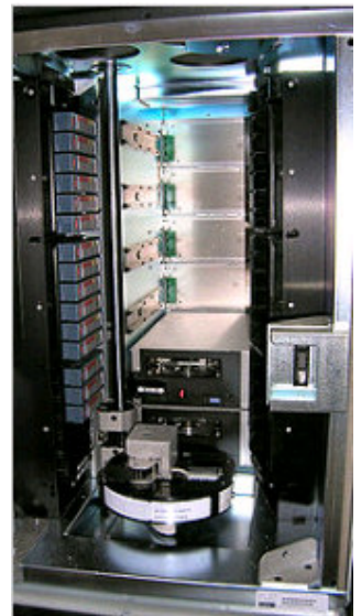
Small ADIC Scalar 100 tape library, robot visible on the bottom, two IBM LTO2 tape drives behind it. Empty room for another four drives in the center. Tape cartridges on the left column, right column empty. Visible height is about 70 cm.
